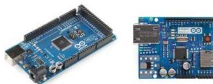
Figura 1 - Arduino Mega e o shield ethernet.
