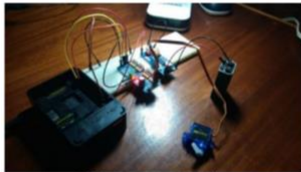
Figura 584 - Teste do Driver PWM com a Raspberry Pi 3
